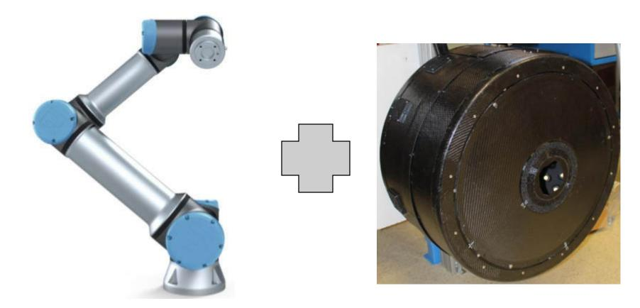
Center of gravity 170mm from the robot head flange Payload 13.95kg
